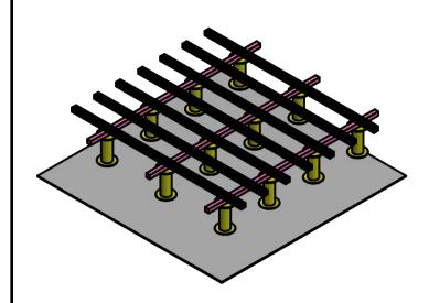
This is a generic example ofd an area of 5.3sqm, with cross frame instalation with pedestals
